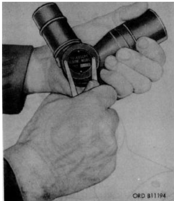
Figure 14. Removal of cover.
